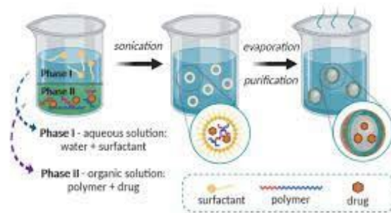
Figure 2: Schematic representation of the solvent evaporation method.
